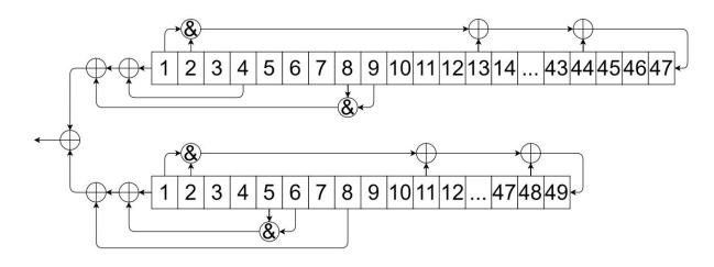
It consists of two shift registers of lengths 47 and 49 with non-linear feedback functions. The contents of the cells of a specific register at any time moment t = 1, 2, ... form the state number t of this register. At time t, each register first generates keystream bit number t and then transitions to the next state number t + 1. The states of the registers at moment t are denoted as
